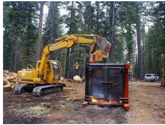
Figure 4: Disposing of forest vegetation in a Air Curtain Destructor, Lake Tahoe Basin Management Unit
